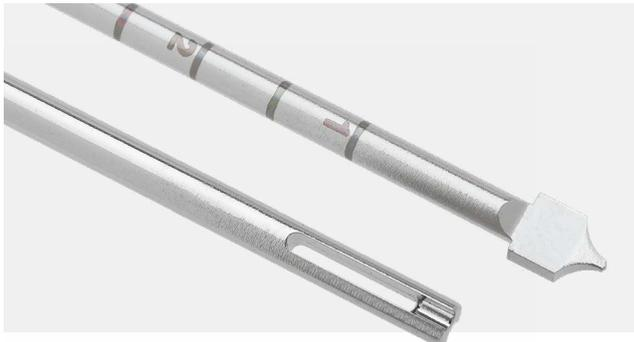
The included TightRope drill pin features a 4 mm spade tip and a closed eyelet with suture recesses for easy passage. The shaft diameter is 2.4 mm. The pin features laser markings in 5mm increments up to 20 cm. The laser marking are calibrated off the trailing edge of spade tip (a.) (Hook the back of the spade on the cortex to measure). The overall pin length 406 mm (16 in).
