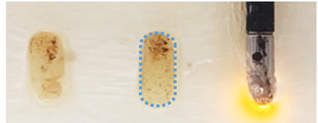
Figure 3. Example Topographical Scan (Left) and Sectioned View (Right) of Indentation Volume via Keyence VR-3200
